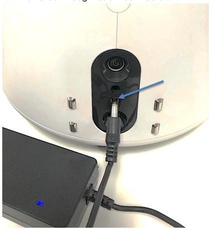
The robot remains functional when it is physically connected to its power supply. It is not recommended to roll the cable as the power jack connector may be damaged.
